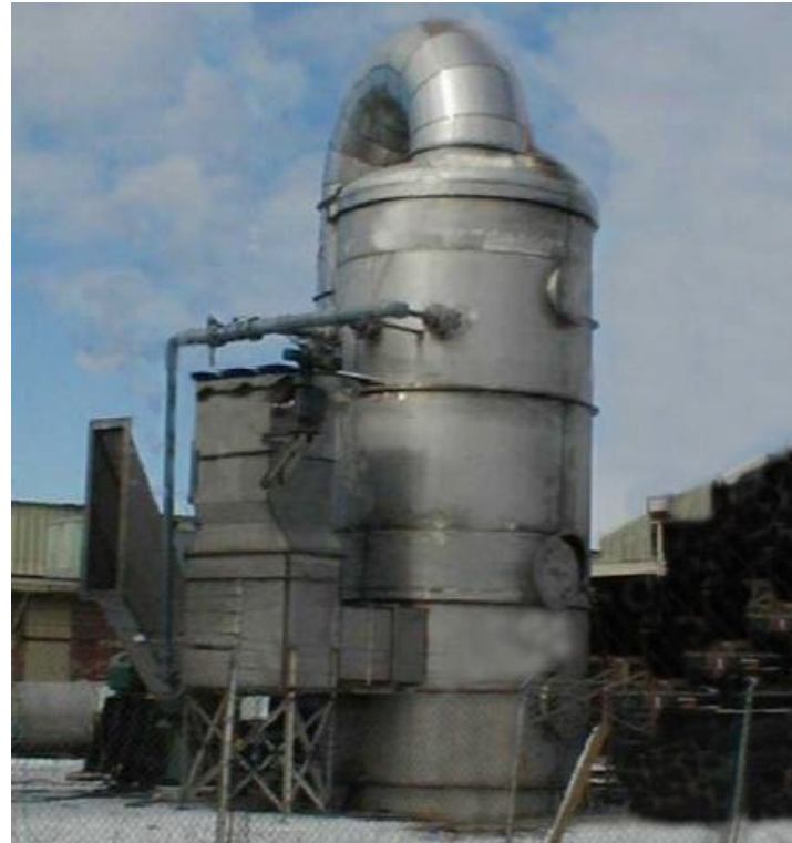
Venturi scrubber used in industry. Note the centrifugal entrainment separator
