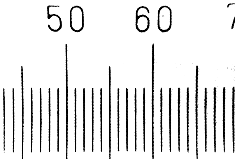
Figure 19.3 Portion of a stage micrometer as it appears at 400\times . Actual distance between the smallest lines is 10\ \mu\text{m} .
