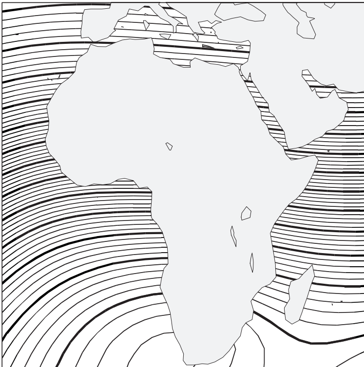
Fig. 5. — Isoclinics along the African coast. Each region of the eastern coastline is marked by a different inclination angle; a similar situation exists for the west coast. Adjacent isoclinics represent differences in inclination of 2^\circ , while dark lines are spaced 10^\circ apart. Isoclinics were derived from the IGRF 1995 model (CAMPBELL 1997) for the year 1995.
