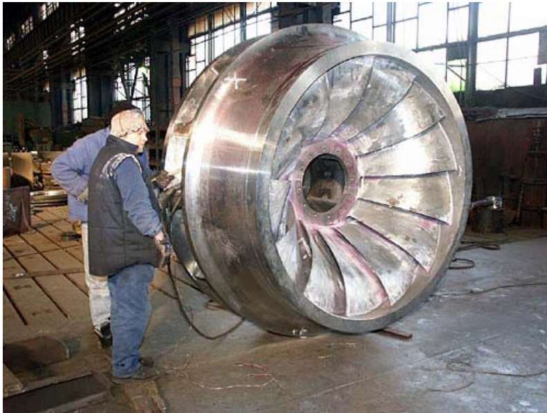
Shiny new Francis turbine
