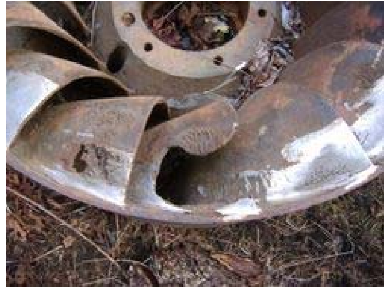
Turbine destroyed by cavitation
