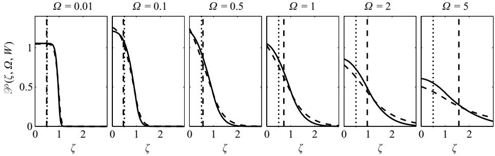
FIGURE 3. PDFs of the positions sampled by matched particles at different values of  $\Omega$  for  $W=1$  (dashed curves) and  $W=8$  (solid curves), with mean sampled positions  $\langle \zeta \rangle$  for  $W=1$  at each time given by a vertical dashed line. The geometric centre of the imaged region,  $\zeta=0.5$ , is indicated by a vertical dotted line.
