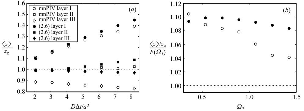
FIGURE 5. (a)  $\langle z \rangle / z_c$  vs.  $D\infty\Delta t/a^2$  for the mnPIV parameters of Li *et al.* (2006) calculated from the PDFs (closed symbols) and artificial images (open symbols, Li *et al.* 2006) for layers I ( $\circ$ ), II ( $\square$ ) and III ( $\diamond$ ). (b)  $\langle z \rangle / z_c$  normalized by  $F(\Omega_*)$  vs.  $\Omega_*$  for layer I (PDFs, closed; artificial images, open), with  $F(\Omega_*)$  given by (4.6).
