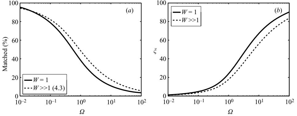
FIGURE 2. (a) Percentage of particles that are matched as a function of  $\Omega$  for  $W=1$  or  $a \leq z \leq 2a$  (solid curve), and by (4.3) for the  $W \gg 1$  limit (dashed line). (b) Average percentage of time-matched particles spend sampling at distances  $\zeta > 1$ , as a function of  $\Omega$ , for  $W=1$  (solid line) and for the  $W \gg 1$  limit (dashed line) computed using (4.2).
