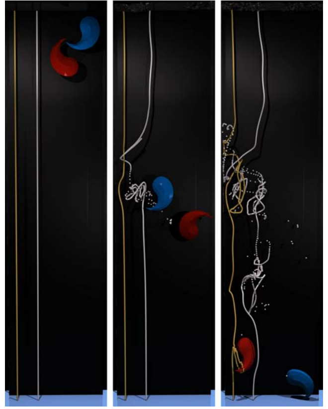
Figure 6: Two odd shaped gems tumbling in a water filled shaft. Passively advected particles mark the fluid movement.
