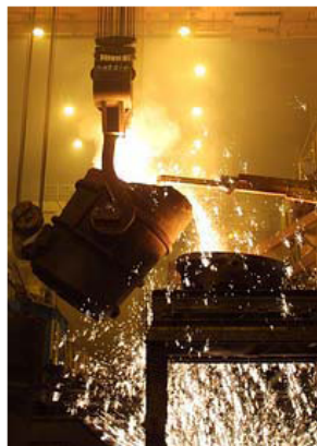
A ladle skims slag off of iron before it is poured into the basic oxygen furnace to be converted to steel.
